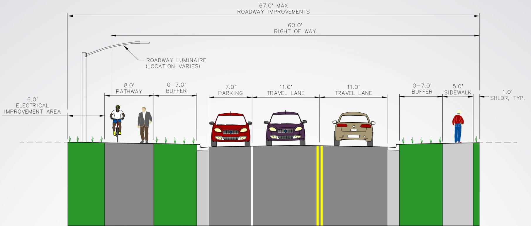
ALTERNATIVE 1 – TYPICAL DCM COLLECTOR ROAD SECTION
